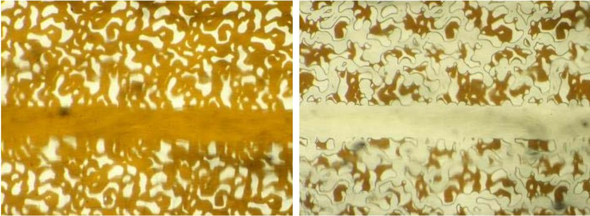
Micromodel (Left : after filled up with oil, Right : after CO2 flooding)
