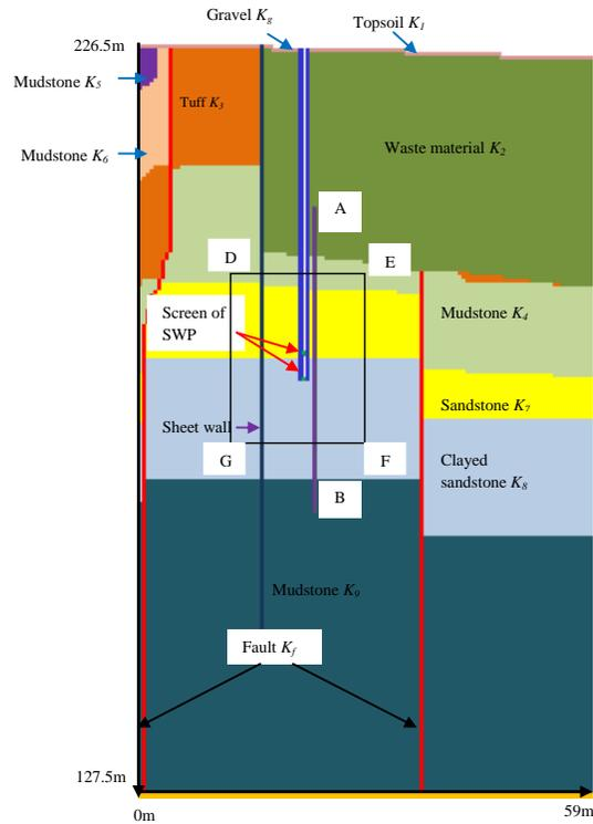
**Fig.4** Geological condition at C-C1
