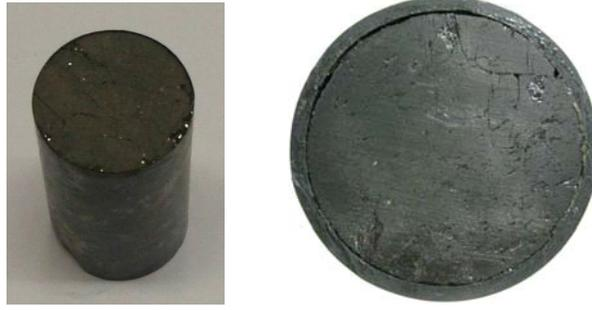
Figure 6: Australian core sample (AU-14) for measuring core strain and permeability
